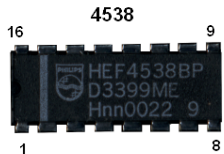
Dual monostable multivibrator
