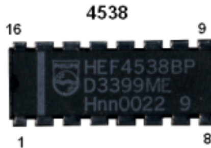
Dual monostable multivibrator
