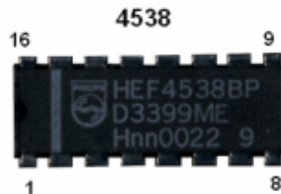
Dual monostable multivibrator
